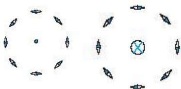
FIGURE 1. The magnetic field due to a long straight current carrying conductor-with currents flowing perpendicular to the plane of the paper outward and inward-the direction of the field lines also change-
