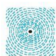
FIGURE 2. Iron filings arranged due to magnetic field of the wire
